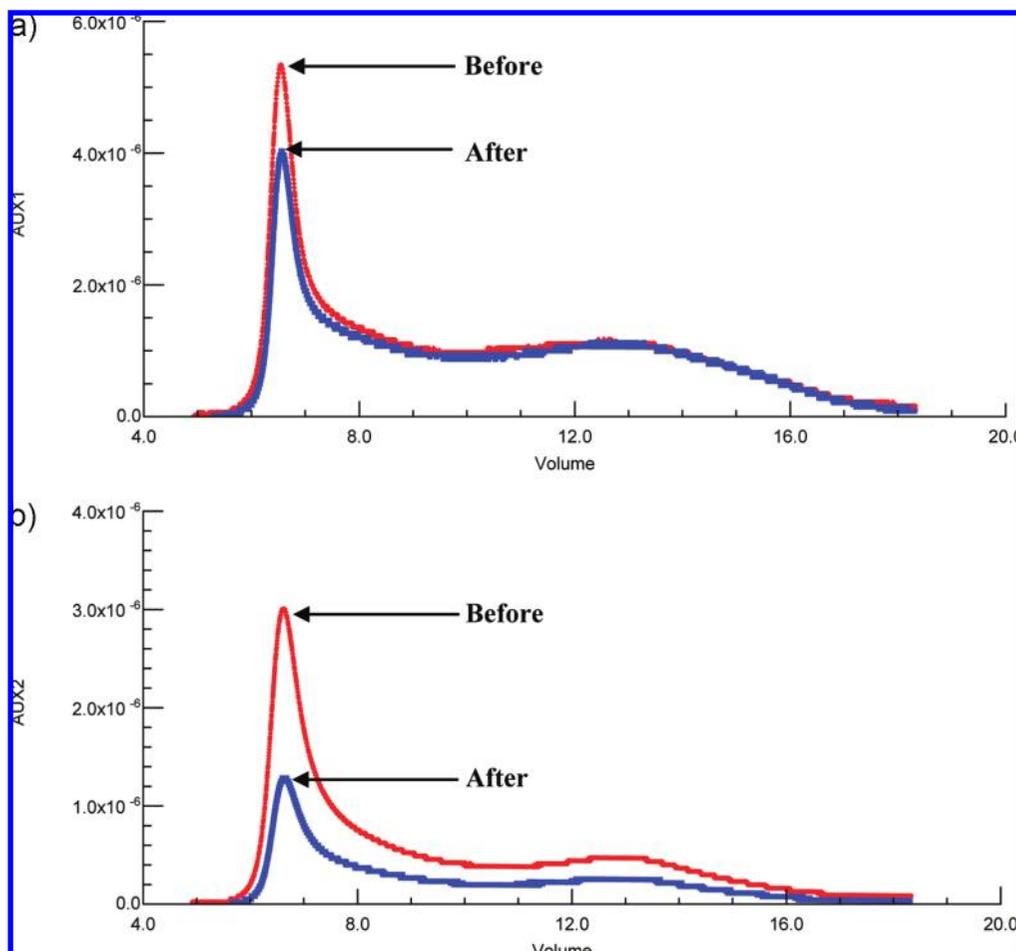
**Figure 2.** (a) RI elution profiles of the SBP sample before and after emulsification with 0.10% w/w initial (before emulsification) polymer concentration. (b) UV elution profiles of the SBP sample at 310 nm before and after emulsification with 0.10% w/w initial (before emulsification) polymer concentration.
