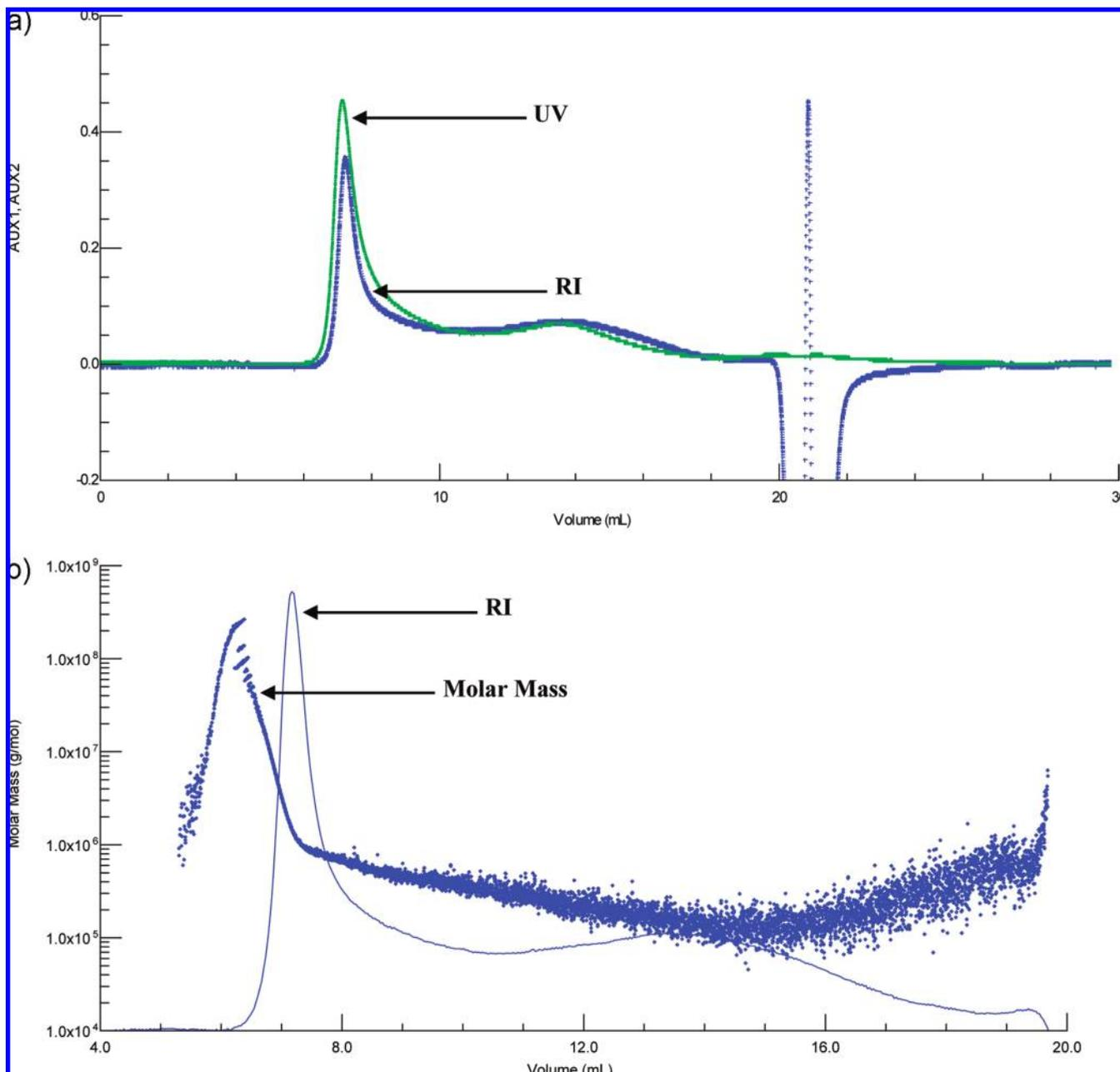
**Figure 1.** (a) GPC elution profile of the SBP showing RI and UV at 310 nm signals. (b) GPC elution profile of the SBP showing RI and molecular mass as a function of elution volume.
