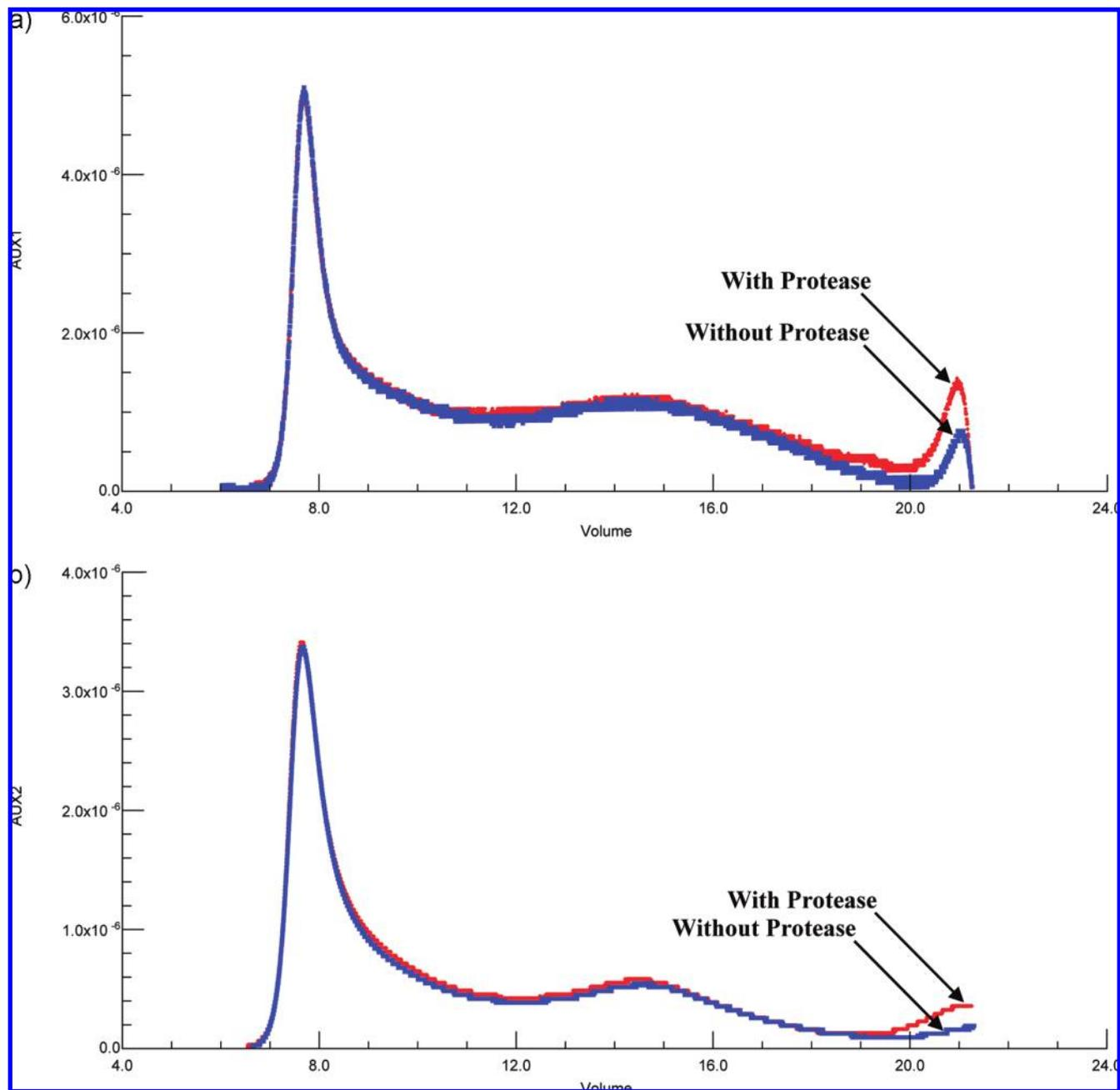
**Figure 5.** (a) GPC RI elution profiles of the SBP with and without protease treatment (46 h). (b) GPC UV at 310 nm elution profiles of the SBP with and without protease treatment (46 h).
