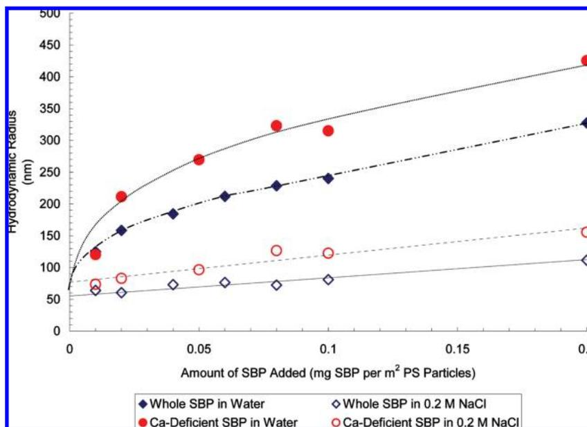
Figure 7. Hydrodynamic radii of the whole SBP and the Ca-deficient SBP in water and in 0.2 M NaCl.
