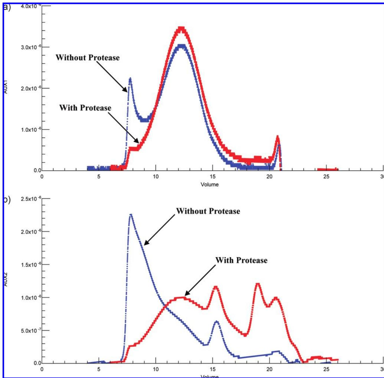
**Figure 6.** (a) GPC RI elution profiles of the GA with and without protease treatment (52 h). (b) GPC UV at 214 nm elution profiles of the GA with and without protease treatment (52 h).
