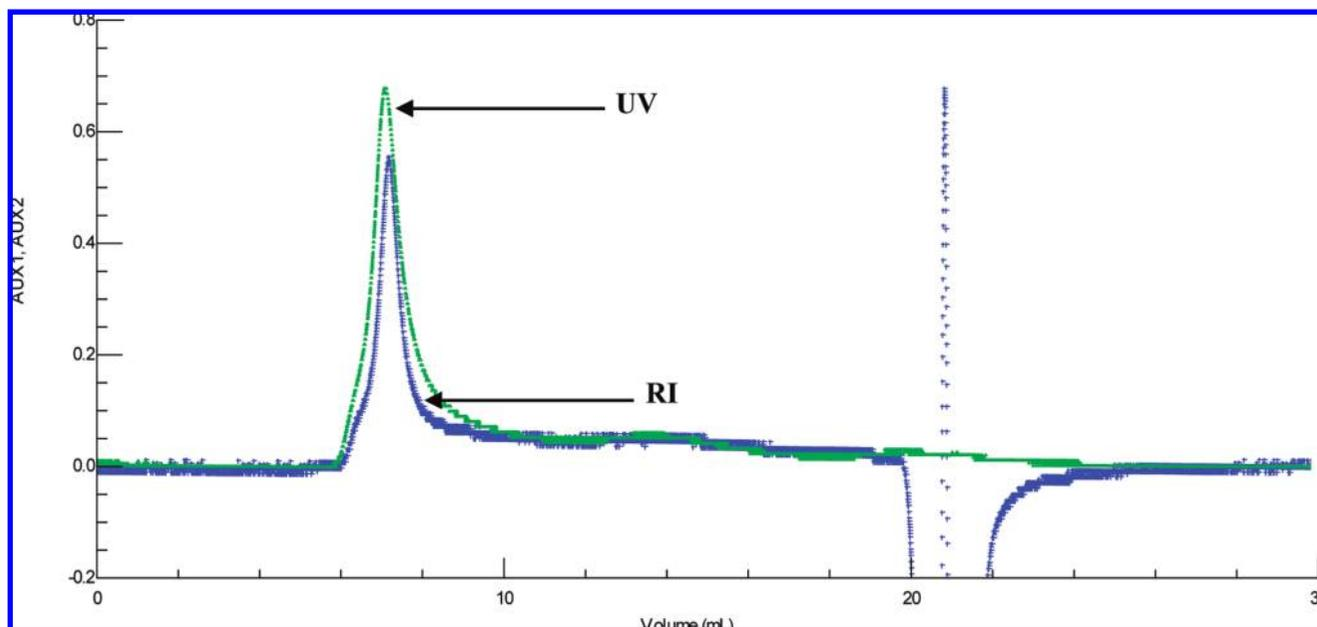
Figure 3. RI and UV (310 nm) GPC elution profiles of the adsorbed SBP fraction.
