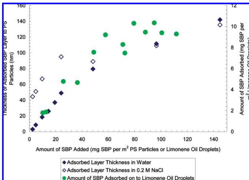
**Figure 9.** Thicknesses of adsorbed SBP layer on polystyrene latex (in water and in 0.2 M NaCl) and the amount of SBP adsorbed onto limonene oil droplets.
