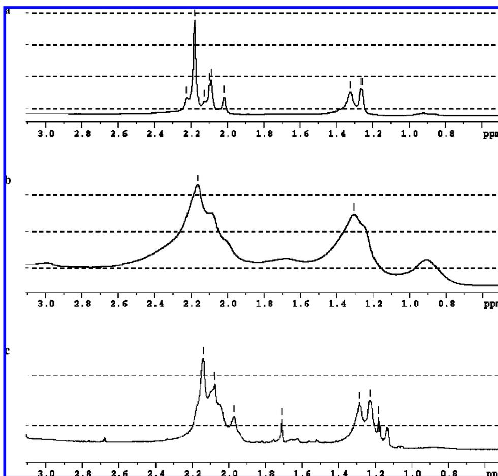
Figure 4. Proton NMR spectra of the whole SBP sample (a), the adsorbed SBP (b), and the nonadsorbed SBP (c) fractions.
