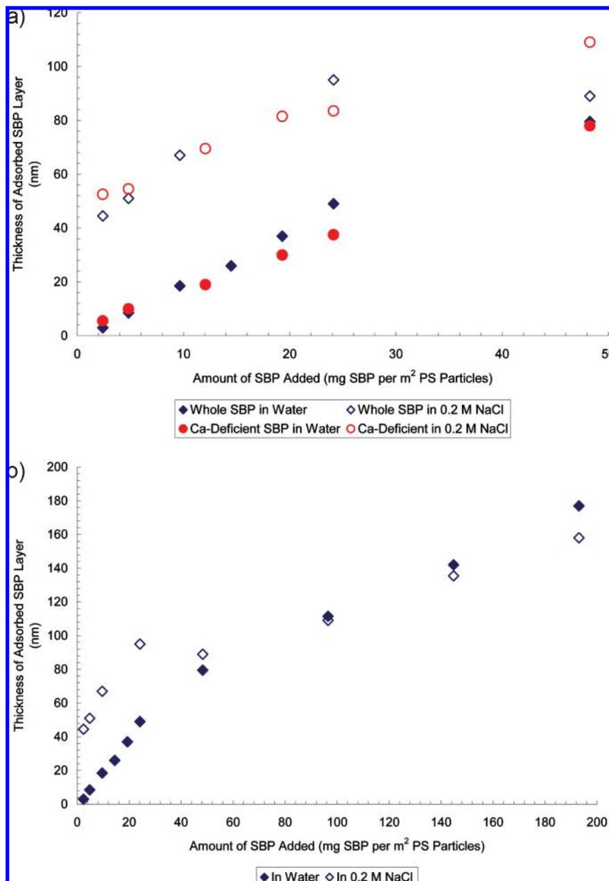
**Figure 8.** (a) Hydrodynamic thicknesses of the adsorbed SBP and the Ca-deficient SBP layers in water and in 0.2 M NaCl as a function of the amount of SBP added. (b) Hydrodynamic thicknesses of the adsorbed SBP layer in water and in 0.2 M NaCl as a function of the amount of SBP added.
